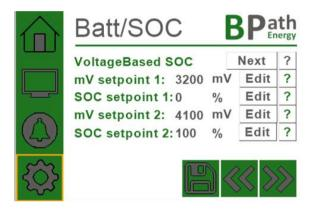
Battery capacity will be estimated based on voltage. This estimation is not 100% accurate but quite good. As the cell voltage is relatively linear to the state of charge.
