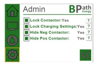
**Lock Contactor:** Allows to lock the contactor setting (see paragraph 2.4.5). Incorrect contactor setting can damage the contactor.
