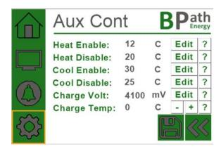
**Heat Enable:** This entry allows to activate a heater, if one is connected. When the average temperature drops below this setting the output will switch high.
