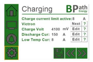
**Charge Volt:** The voltage limit sent to the charger is "Charge Volt" x "SeriesCell".
