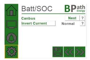
Press "invert current" when direction is not correct. Current drawn from the battery is negative. Charge current is positive.
