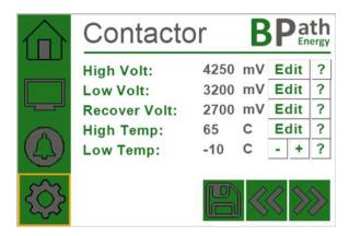
**<u>High Volt:</u>** This command allows entry if the highest allowable cell Voltage. If any cell in any module reaches this voltage the contactor is opened, resulting in disconnecting all devices from the battery.
