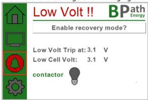
Touch button "Enable recovery mode?" to allow the contactor to close. Charge immediately.
