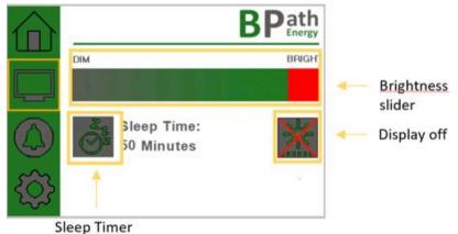
Brightness slider: Move red square from right to left to change the display brightness. Sleep timer: Press symbol and type a value between 1 and 60 minutes to set
