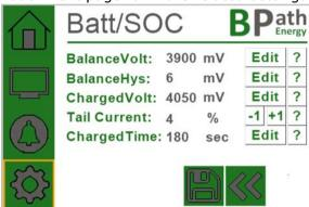
Parameters BalanceVolt and BalanceHys are related to start/stop cell balancing. The cell voltage must be above the BalanceVolt setting to start cell balancing and the difference between highest and lowest cell voltage must be more than BalanceHys parameter.
