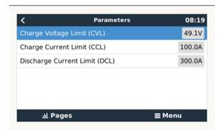
**<u>Discharge Cur:</u>** This is the maximum allowed current drawn from the battery thus used by the inverter. The inverter will stop inverting when the load demand exceeds this allowance.
