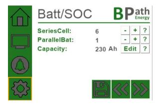
The first parameters on the first page are related. They need correct settings for calculation Voltage and Capacity.
