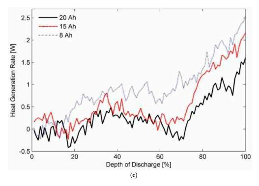
**Figure 6.** Heat generation rates for the three test battery cells during the constant current discharge process at a rate of 1C under ambient temperatures of (**a**) 20 °C, (**b**) 35 °C, and (**c**) 50 °C.
