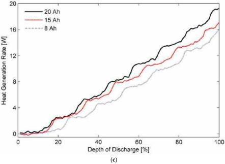
**Figure 3.** Estimated heat generation rates for 8, 15, and 20 Ah LiFePO<sub>4</sub> pouch cells discharged at 3C in ambient temperatures of (**a**) 50 °C, (**b**) 20 °C, and (**c**) 5 °C.
