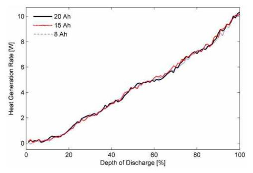
**Figure 4.** Heat generation rates measured for 8, 15, and 20 Ah LiFePO<sub>4</sub> pouch cells in ambient temperature of 35 °C and discharge rate of 3C.
