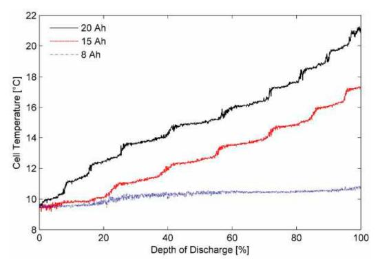
**Figure 1.** Battery cell temperature variation for different batteries discharged using 2C current rate in a sandwich-structured calorimeter in ambient temperature of 10 °C.
