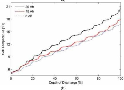
Figure 2. (a) Modified battery calorimeter, markers showing thermal sensor location, and (b) surface temperature variation for batteries of different capacities in modified calorimeter at the ambient temperature of 5  $^{\circ}$ C and discharge rate of 3C.
