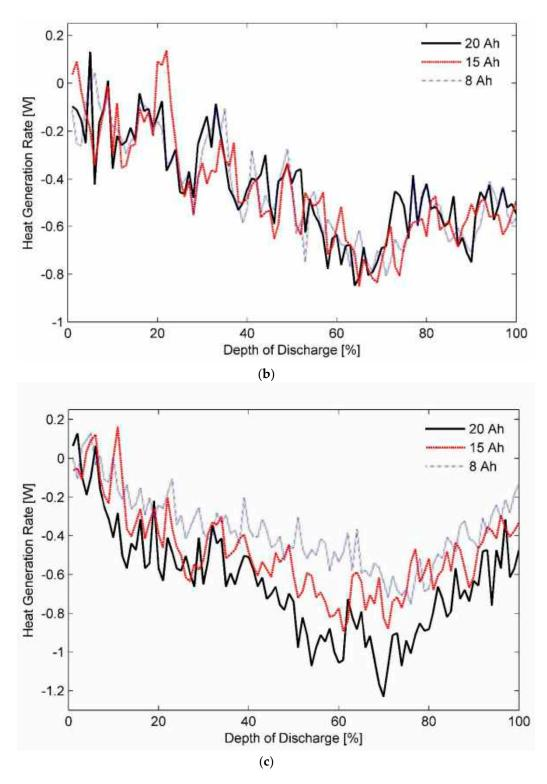
**Figure 7.** Heat generation rates for the three test battery cells during the constant current discharge process at a rate of 0.33C under ambient temperatures of (**a**) 20 °C, (**b**) 35 °C, and (**c**) 50 °C.
