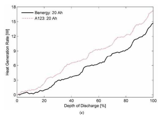
**Figure 5.** Heat generation rates measured for the 20 Ah LiFePO<sub>4</sub> pouch cell (**a**) in an ambient environment of 50 °C for different discharging rates, (**b**) effect of ambient temperature on secondary plateauing at discharge rate of 1C, and (**c**) their comparison with heat generation rates for the A123 20 Ah battery cell at 2C and 10 °C.
